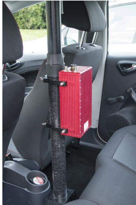
Figure 11. Survey+ mounted on RT-Strut
